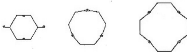
d) Examples of cross sections for steel piles
