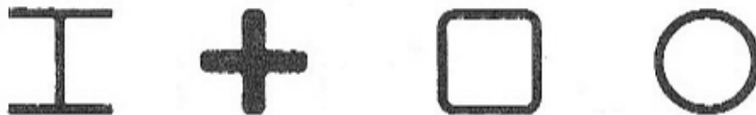
d) Examples of cross sections for steel piles
